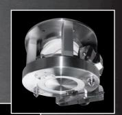
The docking process can be achieved either with a mobile container using a lifting column, or automatically with lifting cylinders mounted directly on to the active valve. After undocking, the active valve will return to its centred position. When redocking, the active valve will pinpoint the passive valve with an accuracy of ± 14 mm.
